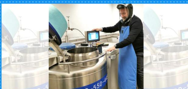
In Manchester, Haier Biomedical has installed a large-scale liquid nitrogen biological sample library for customers, and provides comprehensive management of samples in transportation, storage, processing, and transformation.
