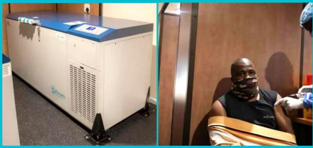
The DW-86W420J is an ultra-low temperature chest freezer with a three-layer sealed structure, the unit is manufactured with three independent inner doors with superior thermal insulation to ensure good temperature uniformity while reducing energy consumption; in addition, the hydrocarbon refrigeration system design is energy-saving and environmentally friendly; while at the same time, it can be connected to the back-up refrigeration system, which has strong flexibility and practicality.
