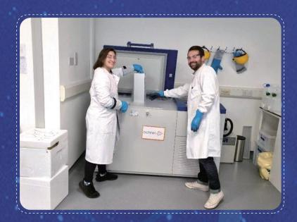
Ochre Bio was one of the first companies to install Haier Biomedical's independently developed -150°C cryogenic freezers. Based on the innovative hydrocarbon refrigeration technology, the product not only offers the lowest power consumption possible (saving energy by 30% around), but it is also safe, quiet (55dB), and suitable for laboratory use. It is a significant step toward reducing the carbon footprint of labs and storage facilities.
